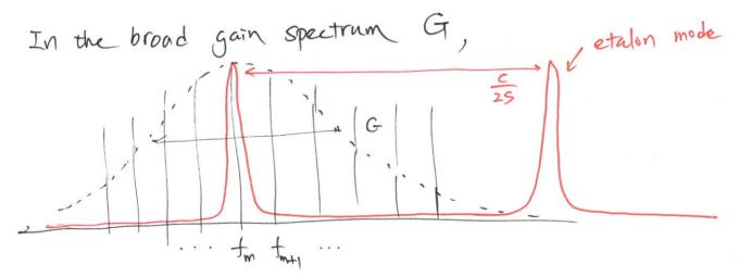
the etalon mode is chossen to pick one mode of the layer cavity, Im.
